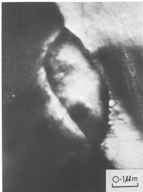
Figure 5 Bright-field electron micrograph showing a grain boundary NiMo particle (specimen aged for 1 hour at 955° C).
